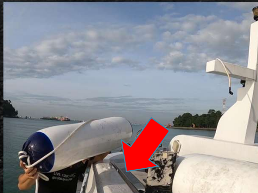
Fenders kept and tied to rail
